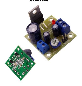
The device is audio amplifier constructed on the base of integral scheme TDA2030. Specifications of the device are: protection from grid noise, high quality sound without a need of preamplifier and easy for application.
